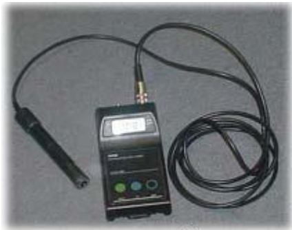
Meter to measure specific conductance in the field and lab
